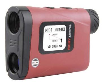
The Closest target model can pick up anda range extremely small or thin targets such as distant power lines and small branches. The Farthest Model displays the distance of the farthest subject-useful when targeting a tree deep in the forest.
